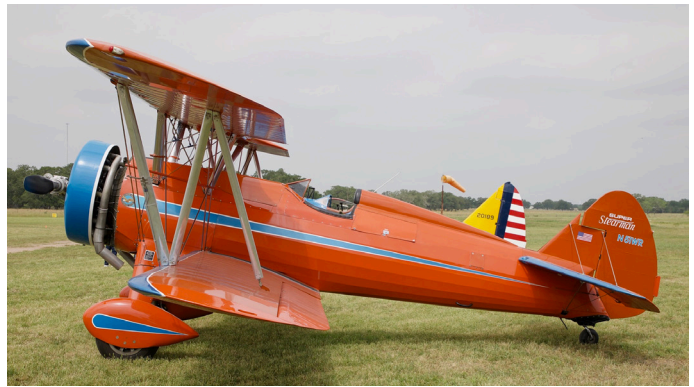
N51WR, Boeing A75N1, msn 75-3660, ff 1942; faired over front canopy; ex USN 37913, N60722, TG-CEG, TG-DUT.
