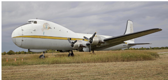
N89FA, Douglas C-54, msn 27249; ex USAAF 44-9023, N88816, XA-MAA, HP-268, XA-MAA, CP-682, N9326R; converted to ATL-98 Carvair (#9 of 21) in 1962, G-ASHZ.
