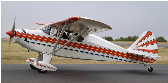
N25TJ, Piper PA-22-160 tailwheel conversion, msn 22-6676, ff 1959.
