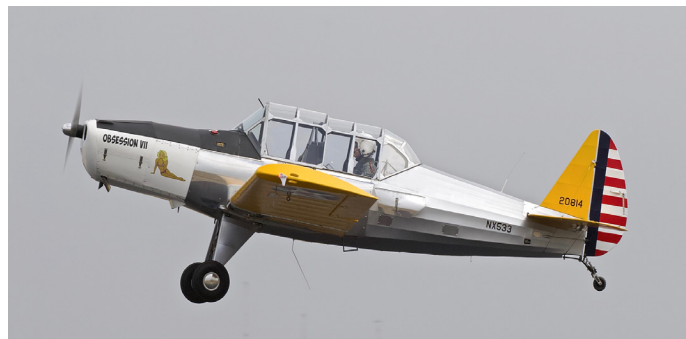
NX533, Spacewalker II/PT-28A (Long, Patrick), msn 20814, ff 2021; w/ T-6 canopy, PT-19-looking fin, and Continental O-200A engine.
