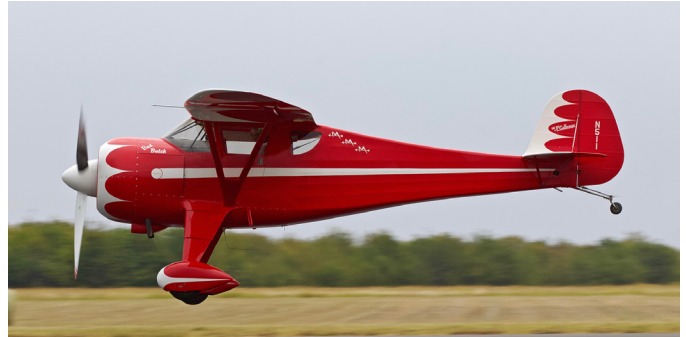
N511, McCullochoupe (Kimball, James), msn MCC1, ff 2004; with Vedeneyev M14P, 9-cylinder, air-cooled radial engine.
