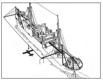
The Brodie System was invented during World War II. A pilot could take off or land with the aircraft hooked to a trolley that ran along a cable. On landing, the trolley provided braking for a smooth stop. The cable and trolley could be rigged on very short jungle fields, or even on ships. This picture shows how a light aircraft could take off or land on a ship using the cable. Image Credit: National Air and Space Museum, Smithsonian Institution NASM-9A001183
