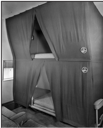
On overnight flights, the 74 seats could be turned into 40 bunks for comfortable sleeping. The bunk beds came with curtains for privacy. On the 24-hour flights across the Atlantic, crew members could conk out on these less luxurious cots.
