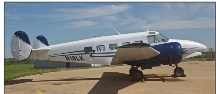
Beech E18S, N18LK, cn BA-230, originally built in 1956, almost certainly as a tail-dragger and subsequently modified.
